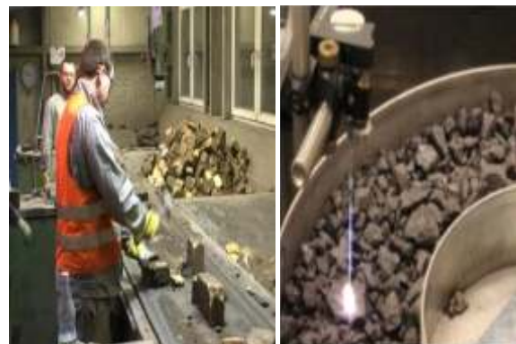
MIRECO employs both hand sorting and laser sorting technology (LIBS)
