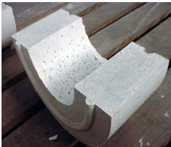
Fig.5: Pre-cast shape for walking beam reheat furnace stator insulation.
