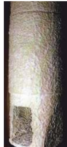
Fig.3: Submerged nozzle with sprayed on microporous insulation on the surface and in the port holes.
