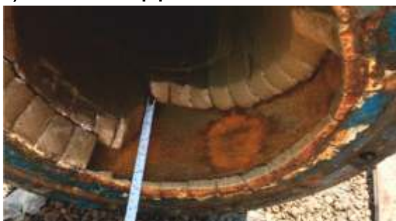
Fig.10 Ceramic tiles dislodged after achieving 3.26 times higher life in horizontal pipe
