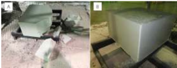
Fig.5: ~400kg blocks after explosion testing at 850°C. A) Fibre-P3 and B) EMSIL-DRY™
