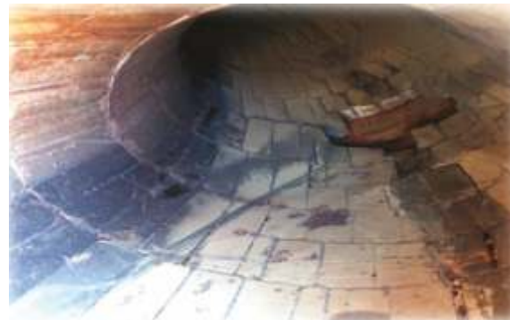
Fig.11 Ceramic tiles dislodged after achieving 4.31 times higher life in bend pipe(bottom)
