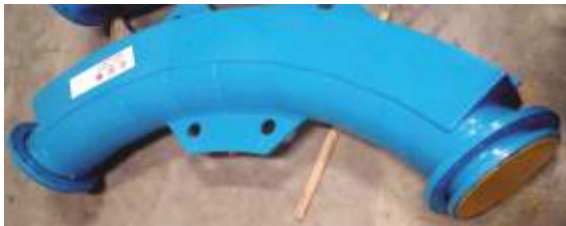
Fig.7 Ejector bend pipe after completion of lining
