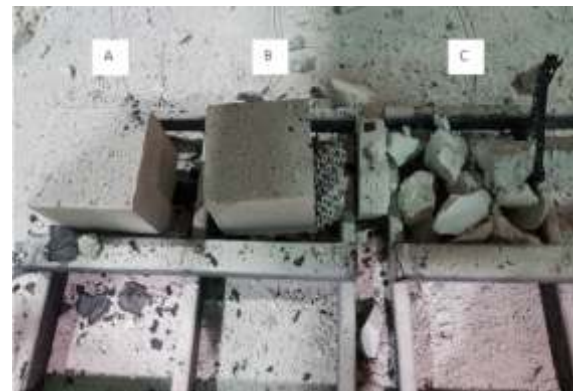
Fig.4: ~80kg (300mm) cubes with different fibres after explosion resistance test (from 20 to 850°C at 50°C/hr). A) Fibre P3, B) EMSIL-DRY™ and C) Fibre-P1. The NCC with Fibre-P2 looked like cube C) Fibre-P1.
