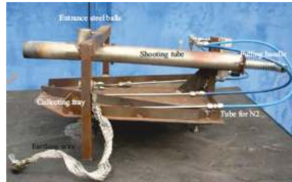
Fig 10: High temperature impact test shooter.
