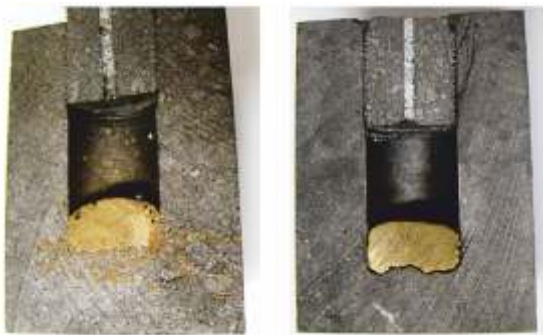
Fig 13: Hot metal penetration test. Left: material penetrated under 1 bar over pressure. Right: material after testing under 2.5 bar over pressure.
