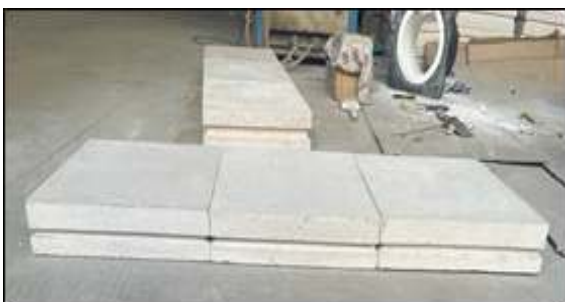
Figure 6: Floor tile after firing and dimension inspection
