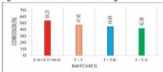
Fig.10: Measurement of slag corrosion
