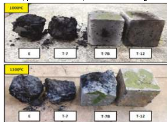
Fig.8: Appearance of the samples after explosion spalling test
