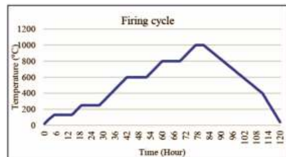
Figure 4: Firing cycle for casted flooring tiles
