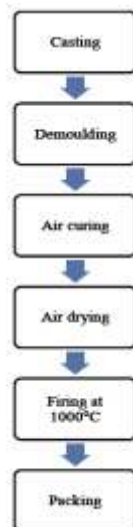
Figure 3: Flow chart for precast manufacturing process
