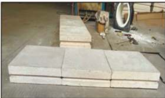
Figure 6: Floor tile after firing and dimension inspection
