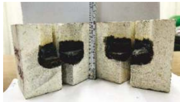
Fig4. Cup slag corrosion test of fired alumina-spinel brick
