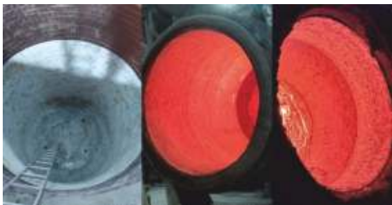
Fig5. Fresh lining (left), preheated lining (middle), used lining towards end (right)
