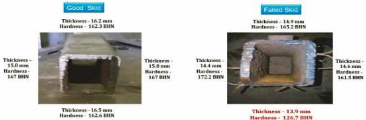
Fig 2-Cross Section of Good and Failed Skid (Hardness and Thickness measurement)
