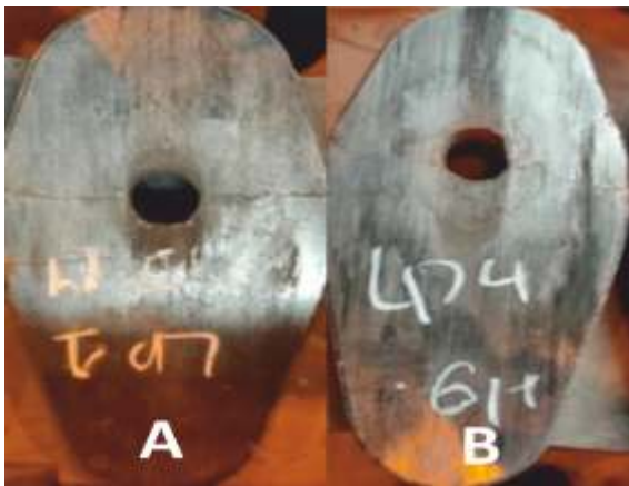
Fig.7 Used plate condition at Plant-Y (A-Standard B- Developed)
