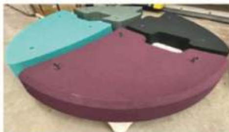
Figure 5 - Styrofoam dummy pieces manufactured to validate the profile of the ladle bottom
