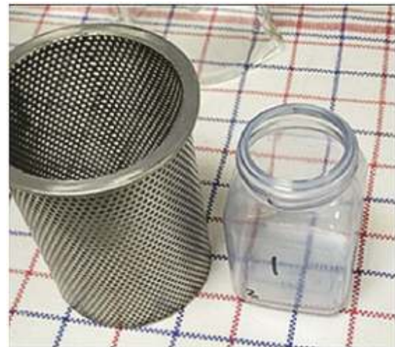
Fig. 4: Basket with plastic container for infiltration of tabular grains by centrifuge.
