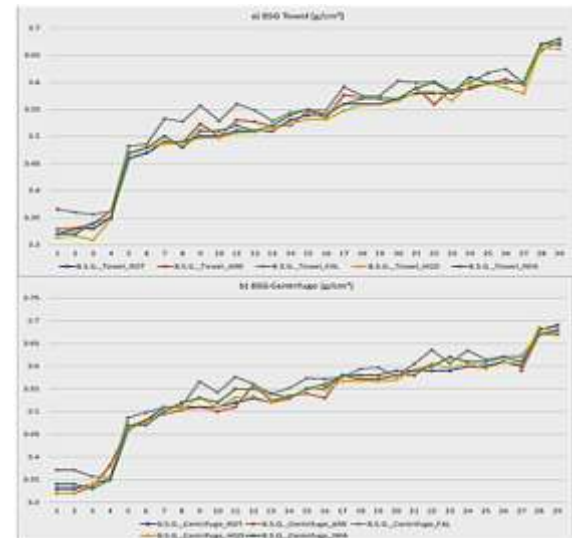
Fig. 7: Bulk density towel (a) and centrifuge (b) results from Gage R&R.
