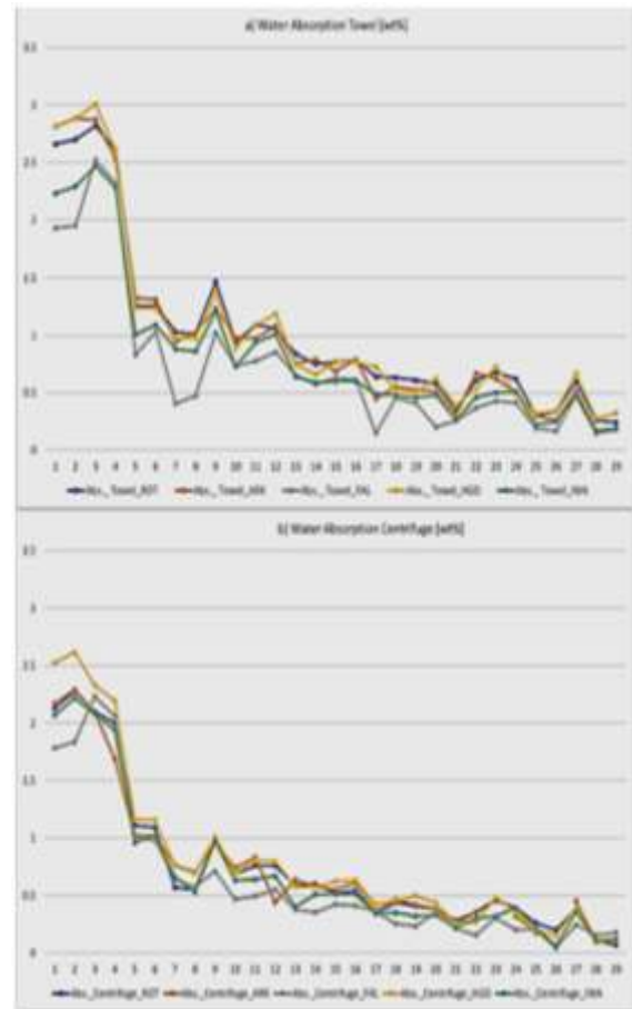
Fig. 9: Water absorption towel (a) and centrifuge (b) results from Gage R&R.
