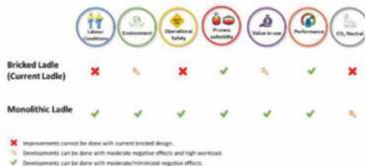
Figure 3 Schematic diagram of improvement opportunities in different areas for bricked and monolithic refractory philosophies.
