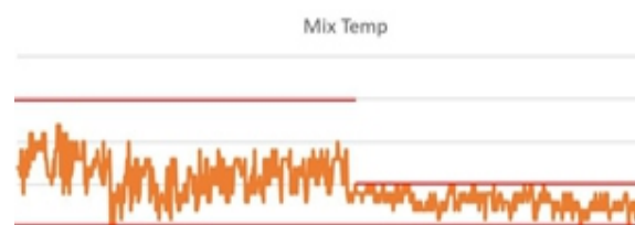
Fig 9: Mix temperature Analysis during manufacturing
